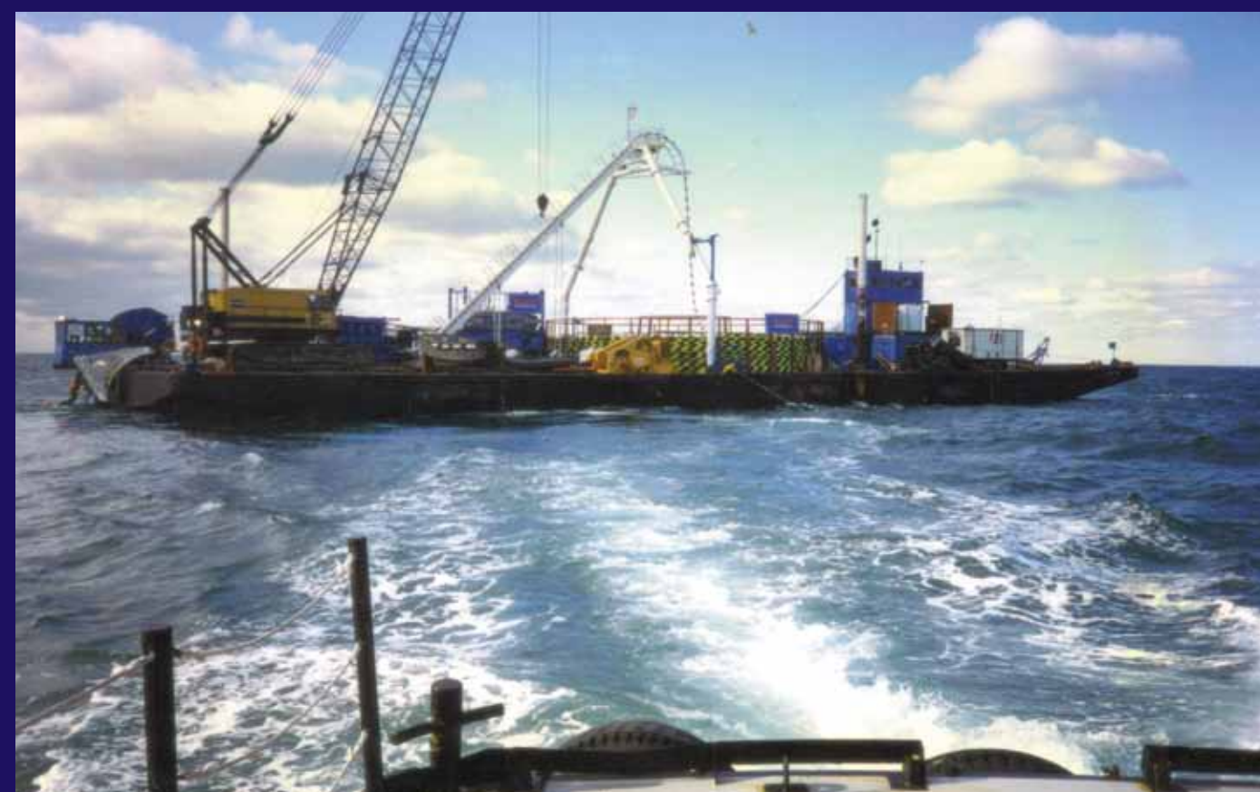
The cable is fed through the plow from a vessel similar to the one pictured above.
